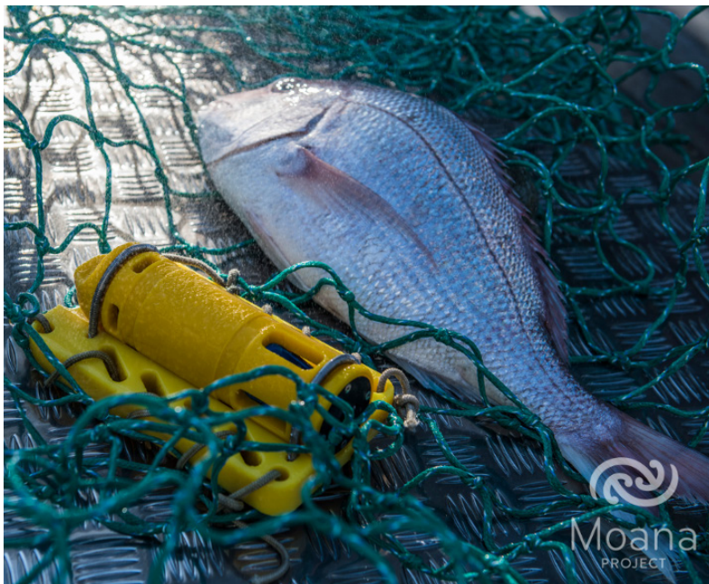
FIGURE 4: Zebra-tech's Mangōpare temperature sensor attached to a trawl net. Moana Project
