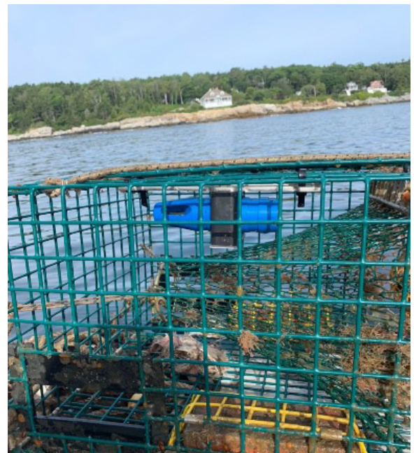
FIGURE 5: A temperature sensor on a lobster trap in the eMOLT project. Jack Carroll
