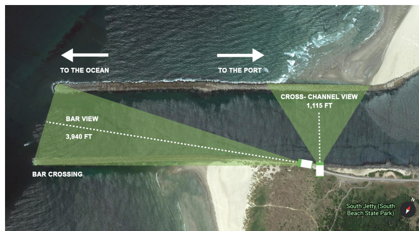
Figure 2. Diagram of the SmartPass setup in Newport, OR using one camera for the “cross-channel view” and one for the “bar view.”
