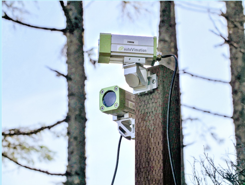
Figure 5. Example of two-camera system. Each imaging sensor was rated for operating temperatures between 0 and 45 degrees Celsius, with a storage temperature between -30 and 60 degrees Celsius, and was powered via Ethernet which allows for the sensor to be deployed 100 meters away from the recording computer without any extenders. Each sensor and associated optics were installed in a waterproof housing which protected against dust and sand; these protections were critical, given the damp, cold weather that dominates the Oregon coast for much of the year.
